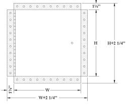
ROUGH WALL OPENING IS DOOR SIZE + 1/4" OR + 6MM \*NOT AVAILABLE FOR CEILING RATING (MAXIMUM 24"X36")
