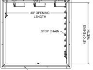
Ø 7/16 MOUNTING HOLES AROUND ENTIRE PERIMETER SPACED 18-24 O.C.
