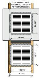
A premium flush mount exhaust fan cover for a 14" x 14" drywall opening. This cover can also be used as a cold air return, and yields a 12.25"x12.25" accessible area.
